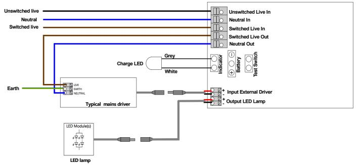
Note: Lamp and driver plug and socket may be opposite gender or different type. Observe emergency module label information for wiring!
